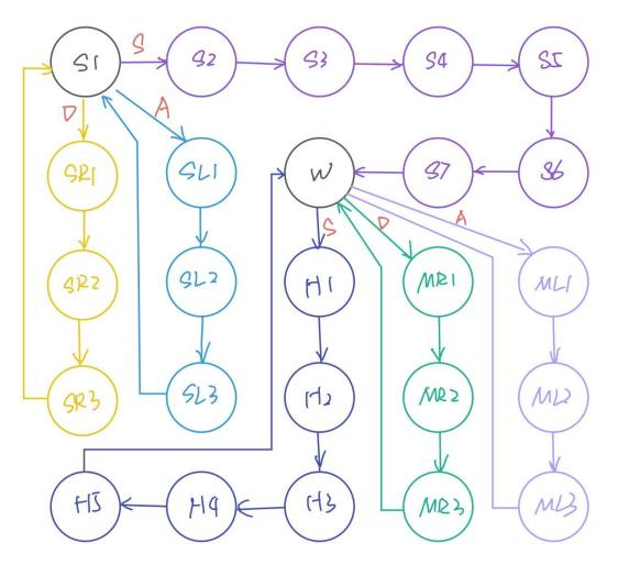
Although there are 25 states here, we actually have 17 states pictures since some states share one picture. Move left and move right can use the same three states' picture but with opposite directions. I first calculated the states than exported the corresponding part of 17 states picture, this can help me save much more memory than if I use 25 different pictures to read. The following algorithm will give the relative read address for our choice of state.
